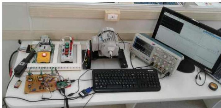
Figura 3 – Bancada experimental HIL.
